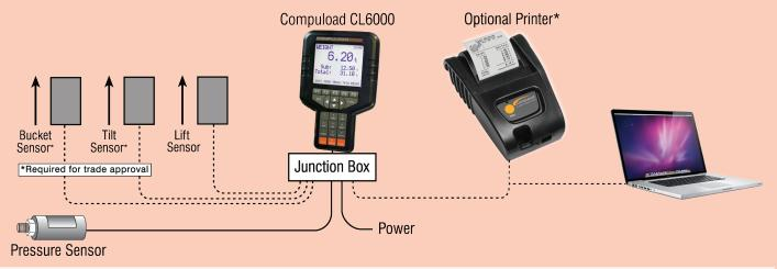
The Compuload CL6000 is a fully electronic modern scale ideally suited for use with Front End Loaders, Skid Steers, Tele Handlers, Container Lifters and Forklifts. Available in two option set ups.
